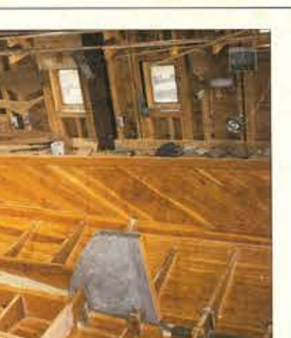
Top left: Having planked up the boat upside, Dr Chile Crisler and friends turn it over for fitting out.
